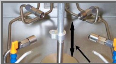
Gas & Air Application with Torch Oscillation *
